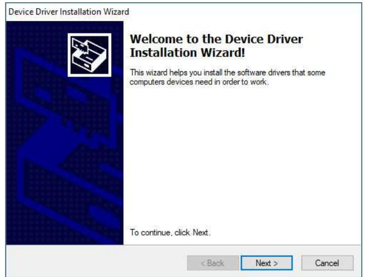
8. Allow the device driver installation to run. Drivers will display as Ready to use when installation is complete. Click Finish.
