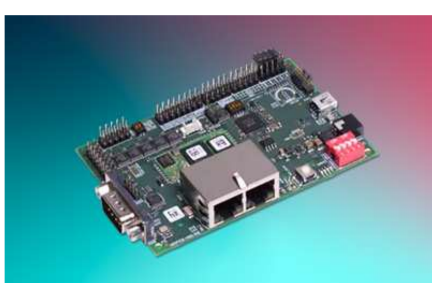
NRPEB H90-RE: netRAPID H90 Evaluation Board - Real-Time Ethernet & Fieldbus:
