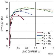
**36VOUT Efficiency** 100 95 90 EFFICIENCY (%) 85 80  $V_{IN} = 12V$ - V<sub>IN</sub> = 18V 75  $---V_{IN} = 24V$ ---V<sub>IN</sub> = 36V 70 I 0 0.3 0.6 0.9 1.2 1.5 LOAD CURRENT (A) 8083 G07
