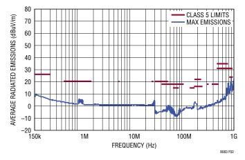
Figure 3. CISPR 25 Average Radiated EMI
