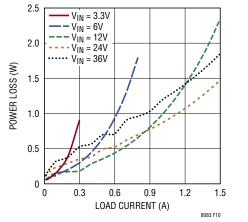
Figure 10. Power Loss at  $12V_{OUT}$
