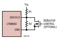
Figure 4. V<sub>IN</sub> Undervoltage Lockout (UVLO)
