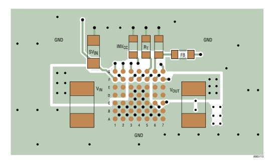
Figure 22. Recommended PCB Layout
