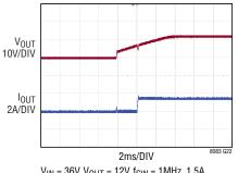
$V_{IN}$  = 36V,  $V_{OUT}$  = 12V,  $f_{SW}$  = 1MHz, 1.5A  $C_{OUT}$  = 10 $\mu F$  CERAMIC SOFT-START CAPACITOR = 0.1 $\mu F$  USE EN/UVLO PIN TO CONTROL START-UP
