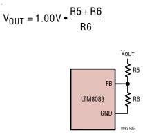
Figure 1. Feedback Resistor Connection
