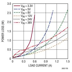
Figure 9. Power Loss at 8V<sub>OUT</sub>
