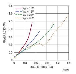
Figure 13. Power Loss at  $36V_{OUT}$
