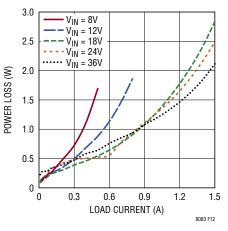
Figure 12. Power Loss at  $24V_{OUT}$
