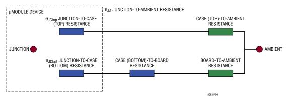
Figure 6. Graphical Approximation of the Thermal Coefficients, Including JESD 51-12 Terms
