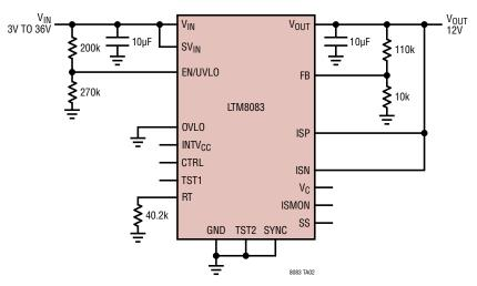
Figure 23. 18W (12V, 1.5A) 1MHz Buck-Boost Voltage Regulator
