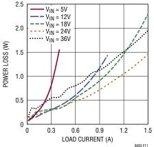
Figure 11. Power Loss at  $18V_{OUT}$
