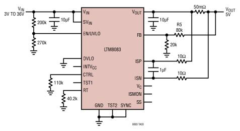
Figure 24. 7.5W (5V, 1.5A) 1MHz Buck-Boost Voltage Regulator with Output Current Monitor
