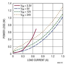
Figure 7. Power Loss at 3.3V<sub>OUT</sub>
