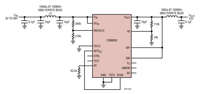
Figure 25. 18W (12V, 1.5A) 1MHz Buck-Boost Voltage Regulator Compliant with CISPR25 Class 5 Limits
