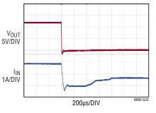
Short-Circuit with 12V\_{IN} and 12V\_{OUT} at  $I_{OUT}$  = 1.5A
