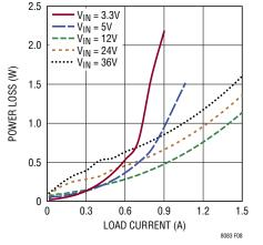
Figure 8. Power Loss at 5V<sub>OUT</sub>
