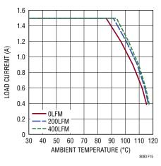
Figure 15. 12V to 5V Derating Curve, No Heat Sink
