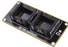
Interface board between the MCU board and up to two Click boards™ via mikroBUS™.
