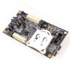
Development platform with an ADUCM4050 ultra-low-power ARM® Cortex®-M4F MCU. Includes accelerometer, temperature sensor and optional Bluetooth LE, LPWAN or Wi-Fi connectivity with an add-on board.
