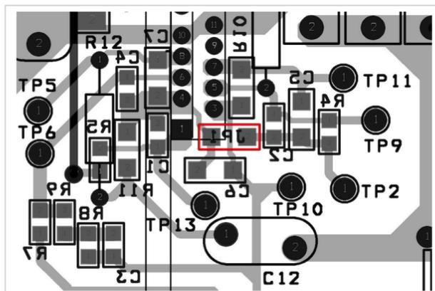
Figure 7: Alternate Layout for LCS Footprint using Round Pads with Jumper Connecting Two Grounds Highlighted.
