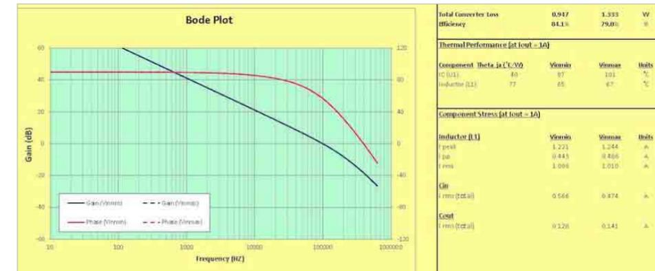
Screenshot of design tool which is a good compromise between high efficiency small solution size and low component cost. The board was designed by the franchised German Distributor Semitron (www.semitron.de) to be used as a replacement for 24V to 5V TO-220 packaged linear regulators which are still in place in many low current indus-
